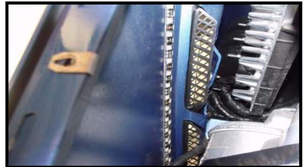
Wipe the mounting area a couple inches away from the vent for best results. Apply the adhesion promotor then peel the backing off the strip and mount it as shown. Its not easy so be patient.
