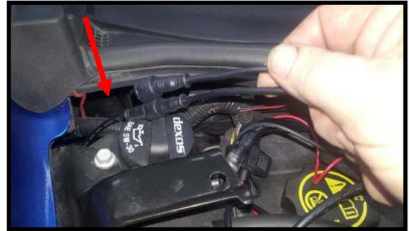
On the passenger side guide the led strip and the extra lead down into the cove area. Use the light as a guide. This shows a Z51 car where it goes behind the oil tank near the coolant tank.
