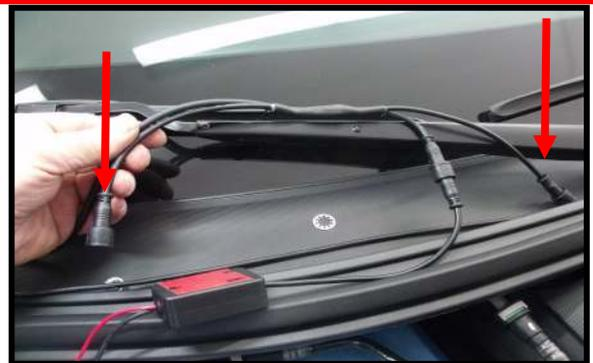
There are 2 leads on the harness near the control box. One is for the hood vent strip and one for the grill strip if used.
