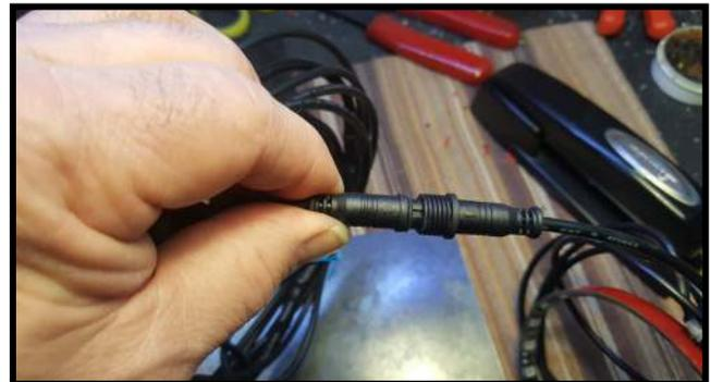
Pull back the nut n the controller connector so you can see the arrows. Line up the arrows and slide the connector together and tighten the nut. Test the lights again.
