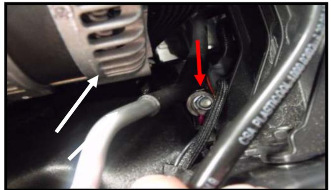
On Z51 cars you can use the 10mm bolt on top of the oil tank for the ground wire. Non Z51 cars, route the black wire along the plastic piping going towards the alternator (white arrow). Secure black wire on the ground terminal below the alternator (red arrow) using the supplied nut. This is where a magnet comes in handy. Its easy to drop the nut.
