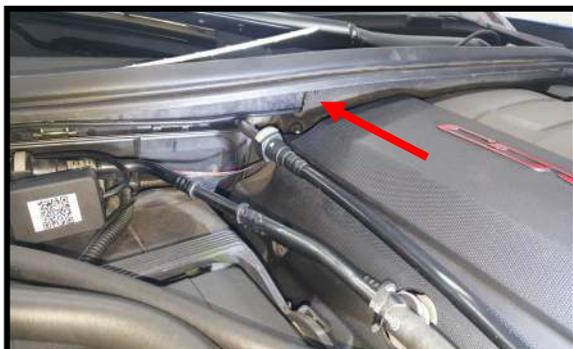
After the strips are mounted you can hide the cable behind the heat shield under the cowl lip on the passenger side. Tuck the cable under the shield all the way over to the drivers side.
