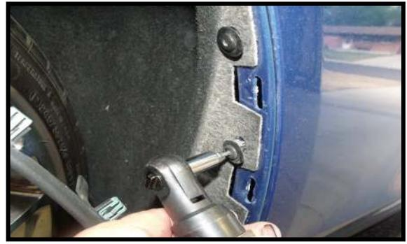
Use a # 15 torx to remove the 3 screws behind the splash shield. Pull back the inner fender panel to get to the cove area. Place a light inside the fender to guide the led strips in place.
