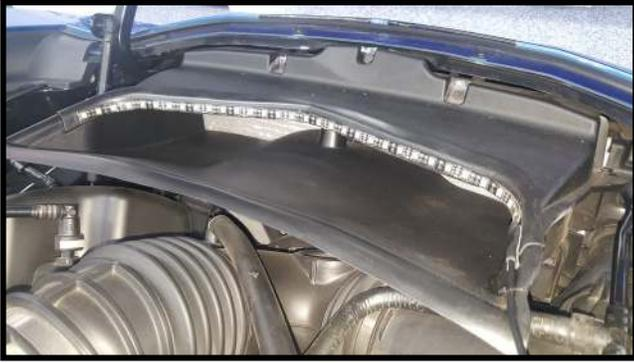
Now you can mount the hood vent strip. Wipe the mounting area with the supplied alcohol pads. Apply the adhesion promoter to the edge of the ducting. Position the strip as shown. Center the strip on the ducting so the wire comes out as shown in the next picture. Be sure to work the strip into the center and corners as this is the most likely place for it to want to pull off. Keep working it until it fits the corners well.
