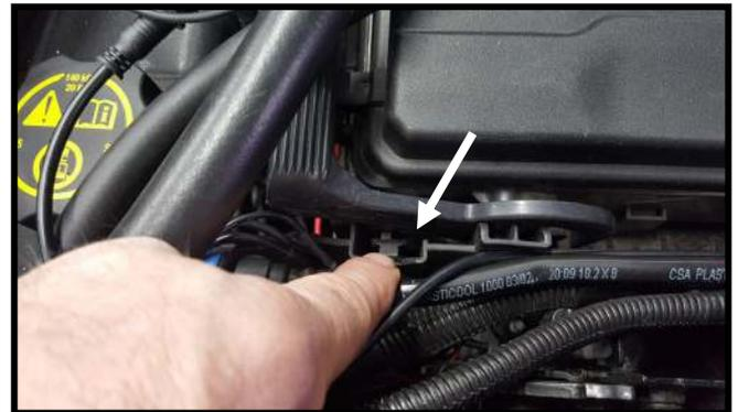
To gain access to the positive connection release these tabs on each side of the rear of the fuse box while raising the handle. Release the cover over the positive terminal
