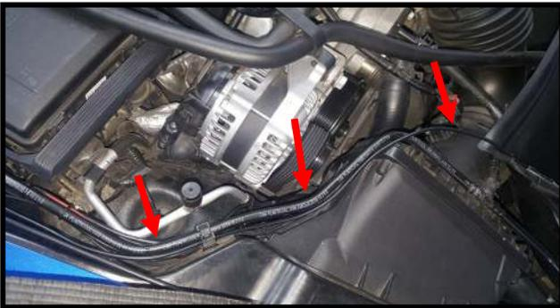
Route the wire along this tubing toward the connectors on the control box. Secure with wire ties.
