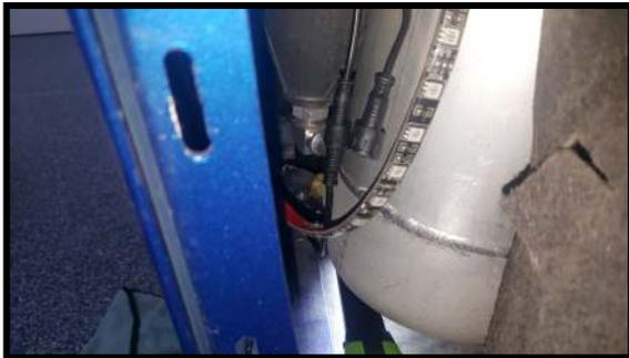
This shows the led strip and extra lead inside the fender cove. The extra lead is to connect the rear fascia kit if you are installing it. Use bungee cords to keep fender shield pulled back.
