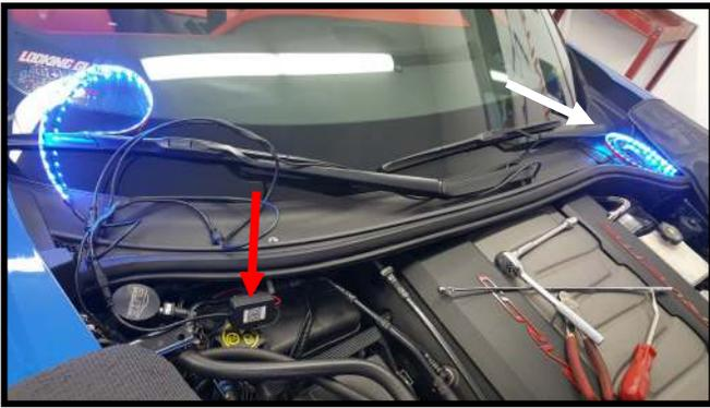
Unpackage the kit and place the remote box close to the fuse box. (red arrow) You can also place it under the hood latch assembly. String the strip with the longest wire across the cowl to the drivers side. (white arrow).
