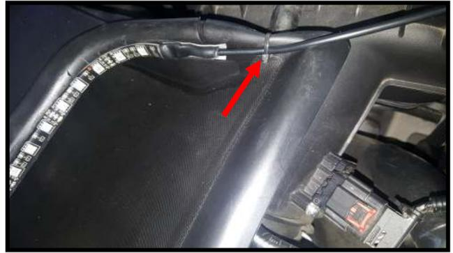
To secure the wire in place drill a 1/8" hole in the ducting below the wire and use a wire tie to secure the wire to the ducting. You can use more than 1 tie if you wish.
