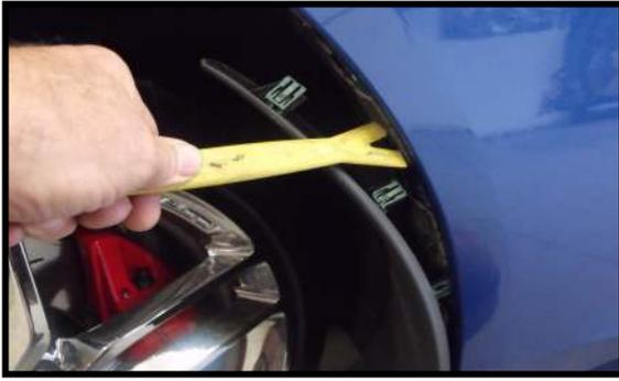
Turn the wheel out on the side you're working on. Use a pry tool to pop the front splash guards out. There is also a screw underneath if you want to take it all the way off. Repeat on both sides.
