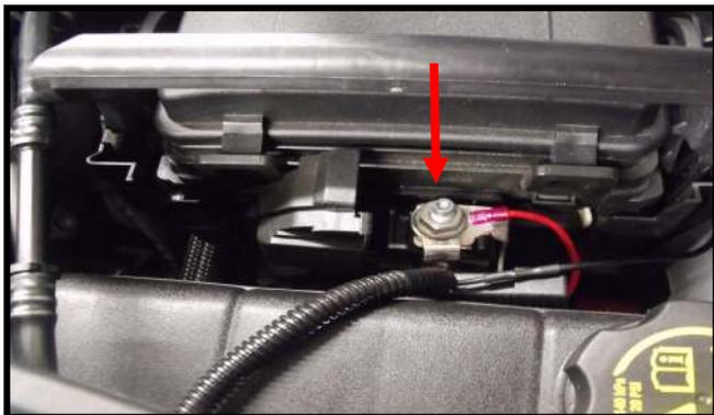
Install the red loop over the positive connection and use supplied nut and tighten. Keep in mind where you want to mount the box and route your wires accordingly. You can re-route them later to hide wires.
