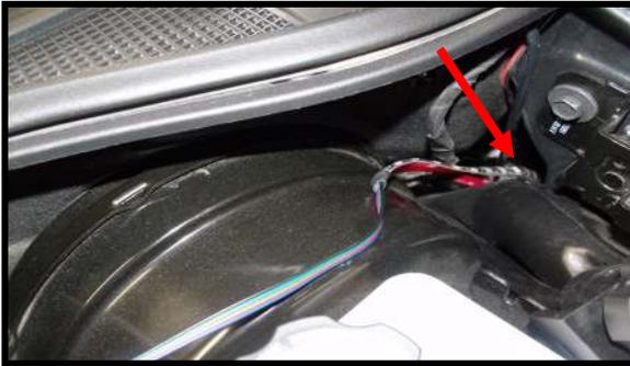
Feed the drivers side led strip past the brake booster and down into the area where you placed the light.
